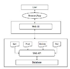
usage of the resources in the server. The note taking system is implemented using MS SQL and Web APIs, which provide low latency communication between client and server, while also implementing efficient caching policies.
