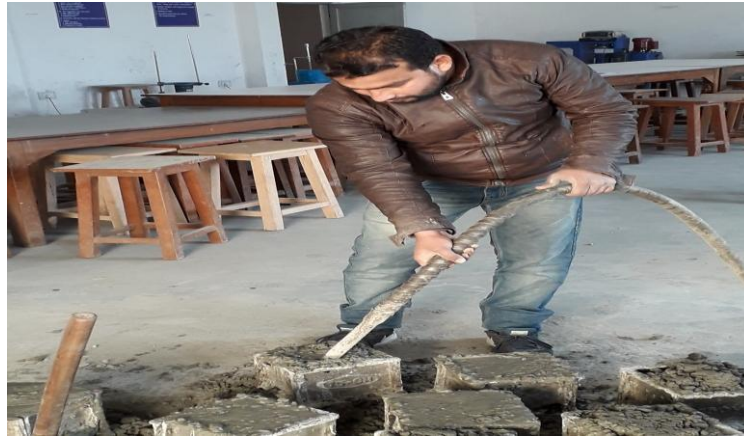
Fig. 3.2 the moulds and vibrating the cube.
