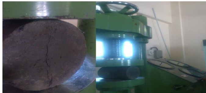
Fig .2 - GEO - POLYMER CONCRETE CYLINDER AFTER SPLIT TENSILE TEST
