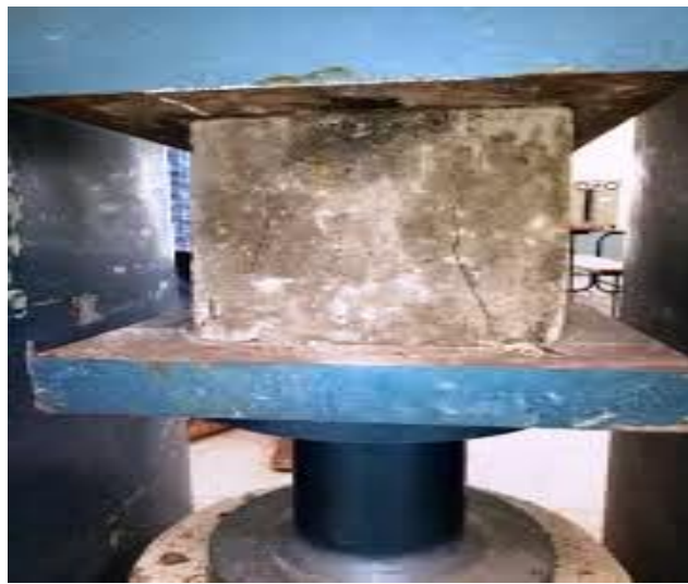
Fig .1 GEO - POLYMER CONCRETE CUBES AFTER COMPRESSION TEST
