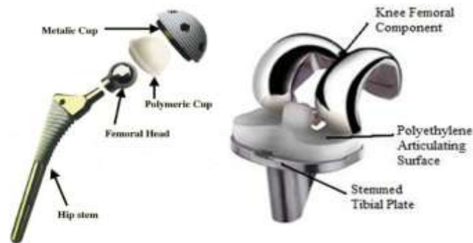
Fig. 11 Schematic diagram of artificial hip joint (left) and knee implant (right) (TitalBestwig Germany)
