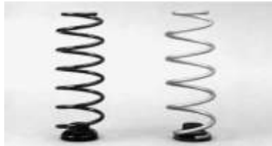
Fig. 9. Rear axle spring of the Lupo FSI (left: steel, right titanium alloy Low Cost Beta [LCB])
